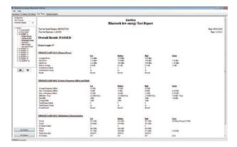
Making Bluetooth low energy measurements on a device with an HCI interface can be fully automated from the [Script Testing] tab.
